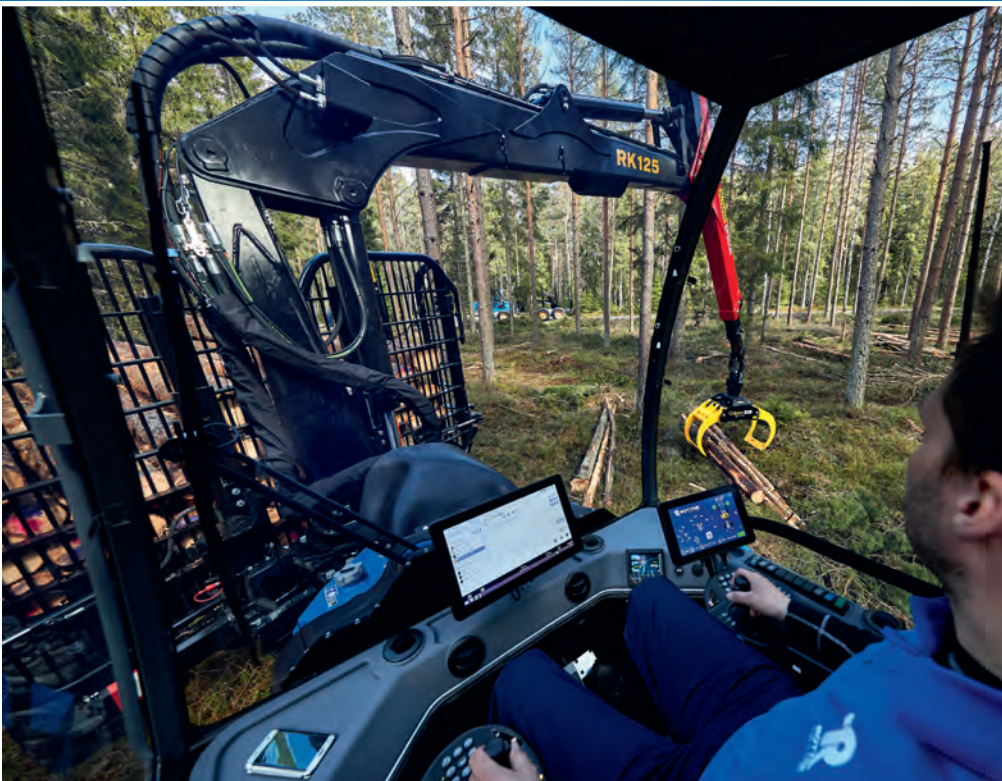
The forwarder cab has an ergonomic operator station with integrated instrumentation and large windows that give excellent visibility.
